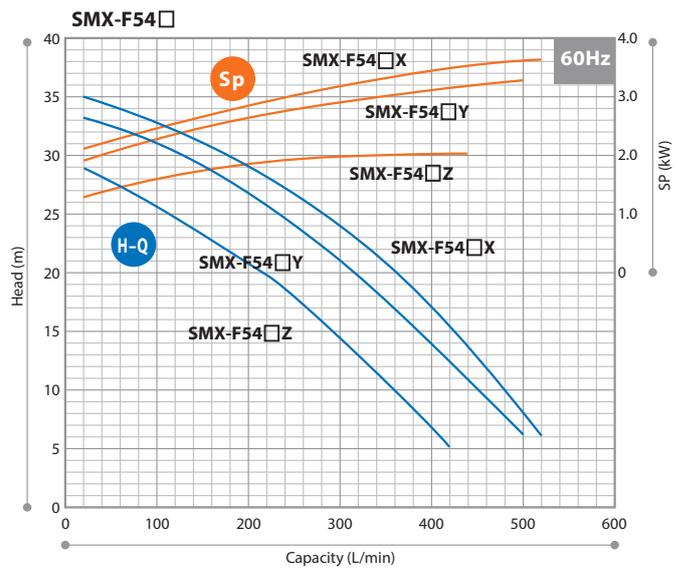
• The shaft power curves shown above are calculated by using our standard test motor. Contact us for detail.
