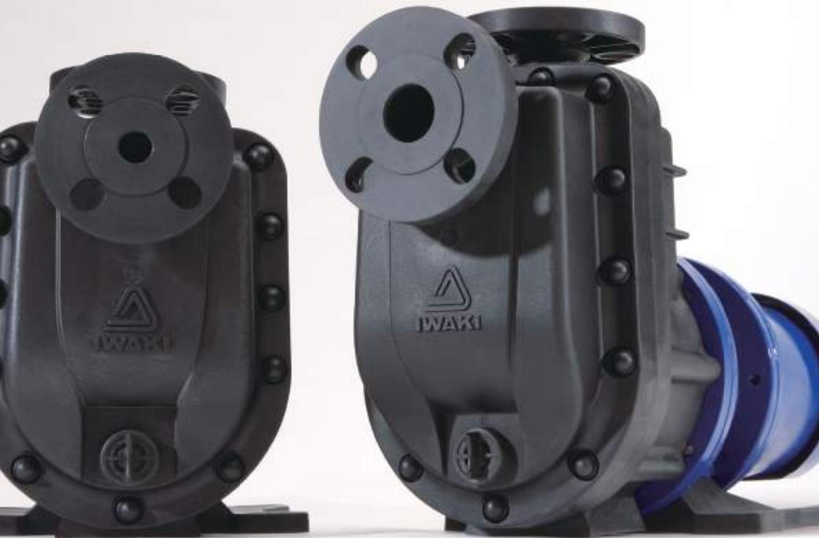
The SMX-F is a horizontal self-priming magnetic drive pump made from fluororesin. Our original self-radiation structure enhances resistance to dry running, cavitation, and closed-discharge operation. In addition, the use of standard motors extends the range of application.
